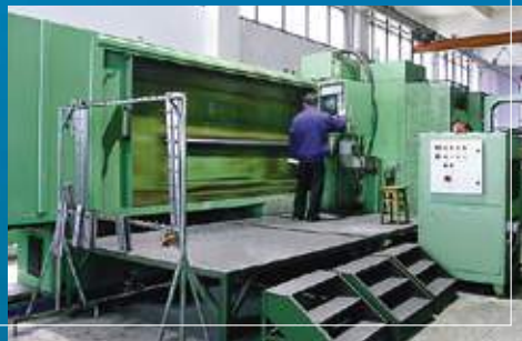
CNC rail grinding machine, 4m, Germany
