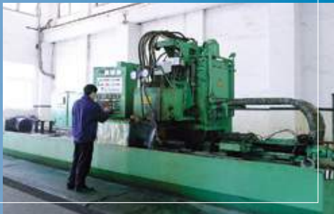
CNC middle frequency quenching machine, 6m, Germany
