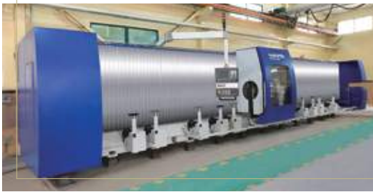
CNC high-speed hard whirling machine, 10m, Germany
