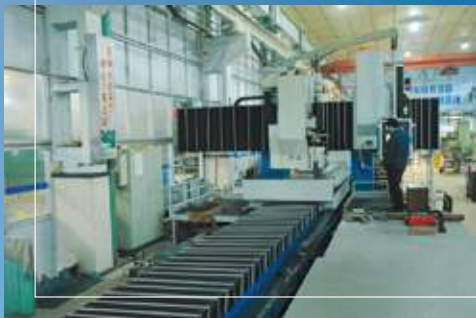
CNC precision plane grinding machine, 6m
