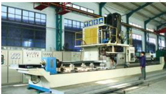
CNC middle frequency quenching machine, 10m
