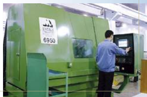
CNC nut grinding machine, England
