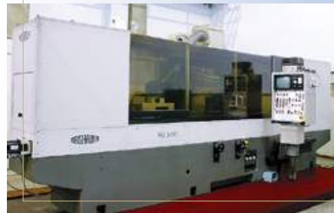
CNC precision thread grinding machine, 2m, Switzerland
