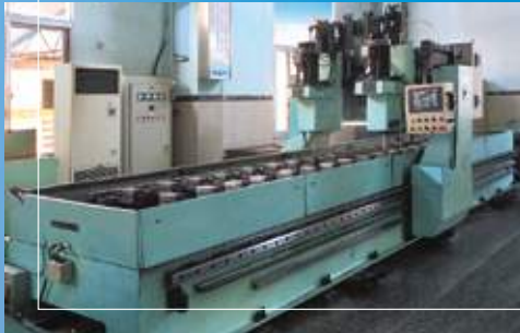
CNC drilling machine, 6m
