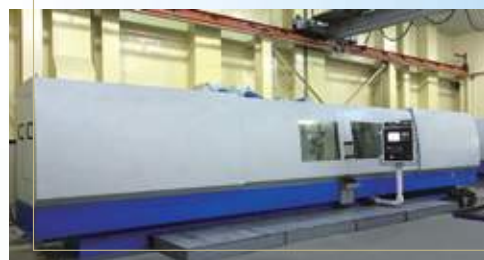
CNC thread grinding machine, 5m
